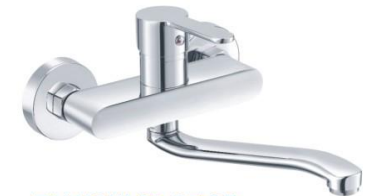
TIANSXL35-05 CP Wall-mounted kitchen Faucet Brass faucet body, zinc handle Ceramic cartridge: dia.35mm Finish: Chrome Plating
