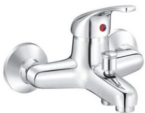
DIWANGH40-03 CP Bathtub Faucet Brass faucet body, zinc handle Ceramic cartridge: dia.40mm Finish: Chrome Plating
