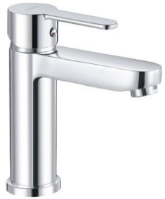
TIANSXL35-01 CP Washbasin Faucet Brass faucet body, zinc handle Ceramic cartridge: dia.35mm Finish: Chrome Plating
