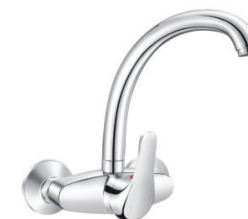
DIWANGH4011012 CP Wall-mounted kitchen Faucet Brass faucet body, zinc handle Ceramic cartridge: dia.40mm Finish: Chrome Plating Central distance: 110mm
