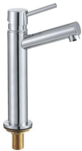
GLG-008T25CP Welded cold Tap Brass faucet body, brass+zinc handle Ceramic cartridge: dia.25mm Finish: Chrome Plating
