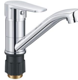
TONGQC35-06A CP Vertical kitchen Faucet Brass faucet body, zinc handle Ceramic cartridge: dia.35mm Finish: Chrome Plating
